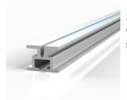
30mm Joist—Used for low buildup areas, but also designed to be bolted directly onto pedestals where a portion of a paved area cannot be supported directly on pedestals. Also intended for steel balconies to facilitate the decking board installation
