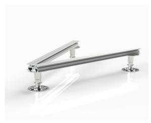
When installing paving on pedestals alone, it is virtually impossible to support the tiles properly in tight corners. Using rails supported by pedestals it is easy to pave into an awkward corner. The Mextru system allows the installer to swap from pedestals alone to rails and pedestals across the area of a site. By maximizing the installation options difficult site can be made easy.
