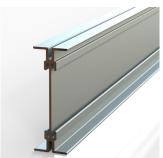
120mm Joist—Used extensively for paved areas that are supported by pedestals or posts. Designed for unsupported spans of up to 1,700mm. Provides slightly better base for paving than the 70mm joist due to it's reduced deflection.
