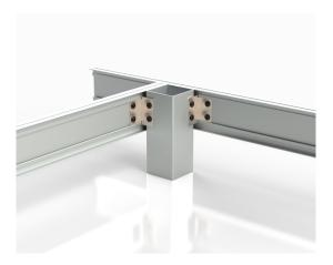
The base structure may also be installed using a post. The structure is bolted directly to the post, which is then concreted into the ground. Providing the ground works are dug to an appropriate depth, the base structure will provide an incredibly solid foundation for either the paving or decking.
