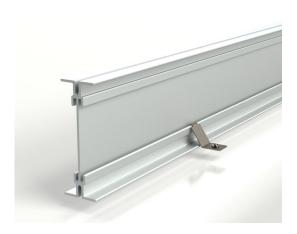
Using the anchor clip to attach the joist directly to an existing substrate. This might be a concrete slab, an existing patio, or onto a brick wall. The anchor clip is deployed either side of the joist to ensure the joist cannot twist.
