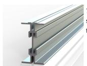
70mm Joist—Used extensively for decked areas that are supported by pedestals or posts. Designed for unsupported spans of up to 1,000mm. Employs the Mextru patented side cleat system for perpendicular jointing of joists.
